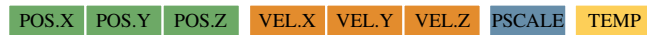
Fig. 8. A particle file stores each particle sequentially as 8 floats: 3 floats for the position, 3 floats for the velocity, 1 float for the pscale (2 times the radius) and 1 float for the temperature.
